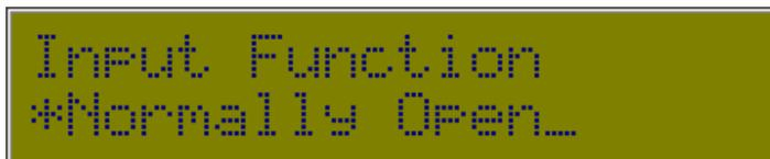
The next setting is the Input Function, which has the currently selected option showing. Scroll through the menu options using <Up> & <Down> to choose an appropriate I/O function, which will be one of the following:
