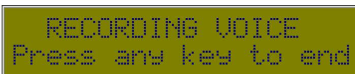
Press any key when you are finished recording. The EDAC700 RTU will play your recording back to you. Press <Ok> to stop listening to the recording playback, then <Ok> to move to the next setting.
