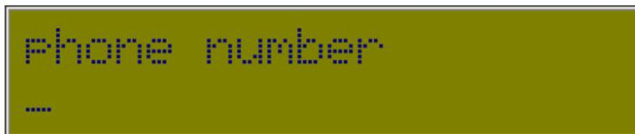
You can now enter a phone number. Do not forget any prefix that may be required to get an outside line, or any required area codes. Use a comma to put in a delay. On an EDAC700 RTU Keypad <\*,> is read as a comma when entering phone numbers.
