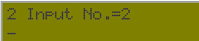
The first setting displayed is the Physical I/O Point number this Input uses. This will be a number between 1 and 20 (unless you have an expansion option). You do not have to use consecutive numbers although it is recommended for simplicity.
