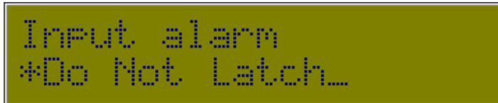
The next setting is the Input Alarm method, which has the currently selected option showing.
