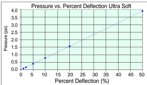
The resultant thickness of the Gap Pad will determine the thermal resistance. Subtracting the initial gap pad thickness by the deflection value, obtained above, will give the resultant thickness. Refer to the graph below to obtain the thermal resistance for a given thickness of material.
